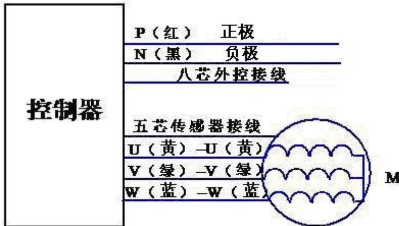
P, N-side DC power supply were connected positive and negative. U, V, W end of the motor three-phase line terminal, respectively, with matching motor leads U (yellow), V (green), W (blue) terminals are connected to the corresponding.
