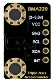
This Triple Axis Accelerometer with Bosch BMA220 is an ultra small triaxial, low-g acceleration sensor breakboard with I2C interface, aiming for lowpower consumer market applications. It allows measurement of accelerations in 3 perpendicular axes and thus senses tilt, motion, shock and vibration in cell phones, handhelds, computer peripherals, man-machine interfaces, virtual reality features and game controllers.
