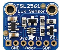
Connect the VCC pin to a 3.3V or 5v power source
